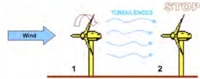
Fig. 2. Wind turbine No. 2 paused to avoid wakes caused by Wind turbine No. 1.
