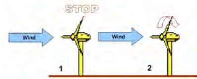
Fig. 3. Wind turbine no. 2 not paused as there is no turbulence.
